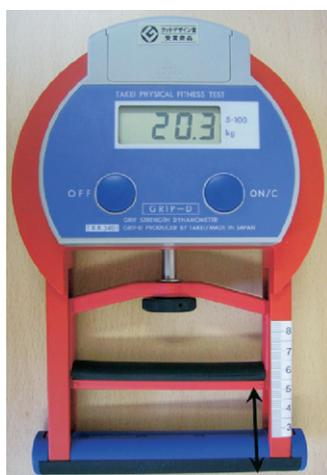
FIGURE 2: Device for measurement of grip span (0.1-cm precision).
